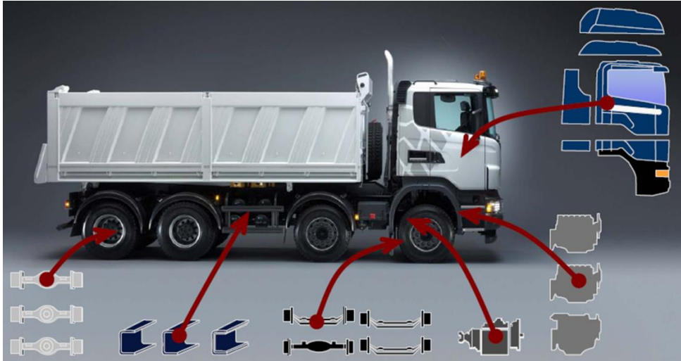
Figure 7:18 An illustration of how the customized truck consists of specific parts, selected among many in the generic product model to generate the product feature that was required.
