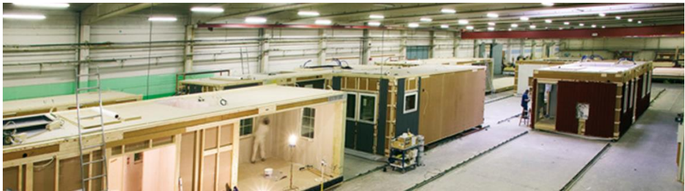
Figure 7:17 The standardized factory line based on highly skilled craftsmen. Some facilitating mechanic tools can be seen to move the 3D-modules within the factory.
