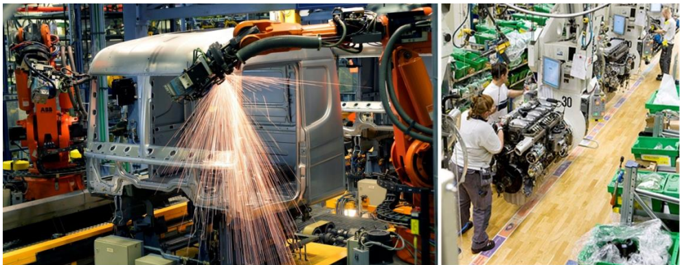
Figure 7:22 Two examples of technology levels. To the left a robot line welding a cabin, to the right manual work in the assembly line motors.
