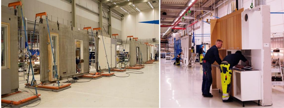
Figure 7:9 Two different assembly lines within the factory that illustrates how each module can have different content and features. To the right the manual work to assemble the kitchen model is showed.
